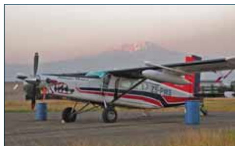
Pilatus Porter PC-6 fixed-wing carrying GT-1A gravimeter. Kilimanjaro looming on the horizon.
